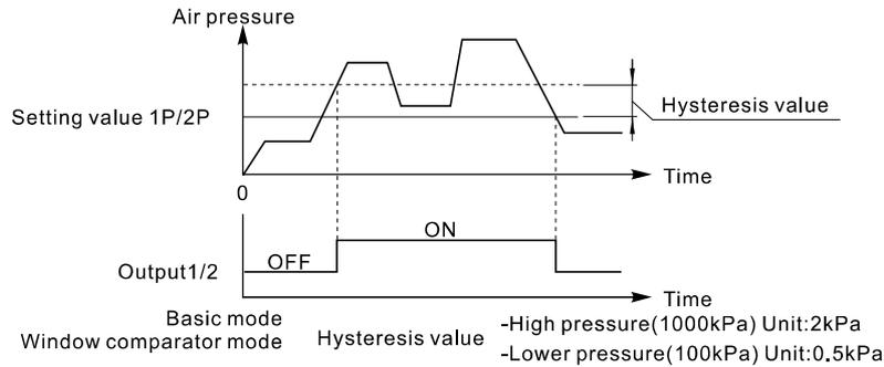
2. Hysteresis mode: Set the pressure value 1H/2H/1L/2L. When the applied pressure value is greater than 1H/2H, the display will ON. When the applied pressure is less than 1L/2L, the display will OFF.
